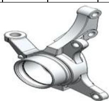
Fig. 10 Part Modelling of Steering Knuckle
