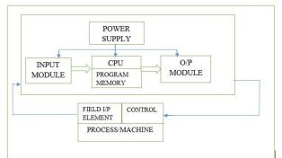
With the coming of microprocessors and associated peripheral chips, the whole process of control and automation underwent a radical change. Instead of achieving the desired control or automation through physical wiring of control devices, in PLC it is achieved through a program or say software.
