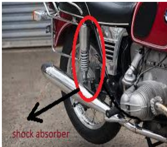
Fig(1) Rear shock absorber and spring of a BMW R75/ 5 motorcycle
