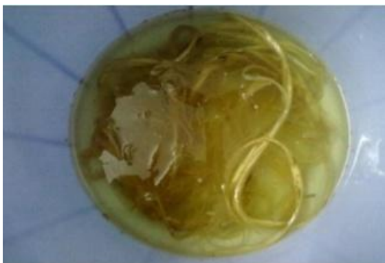
Fig 1: Treatment of Fiber in 2% NaOH solution
