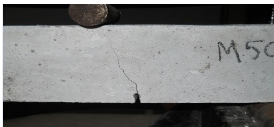
Fig.4.6: M50-Small beam after load
