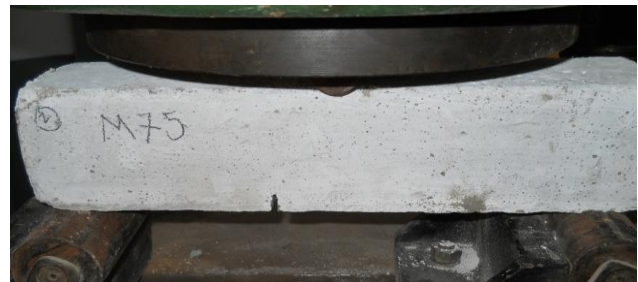
Fig.4.9: M75-small beam before load
