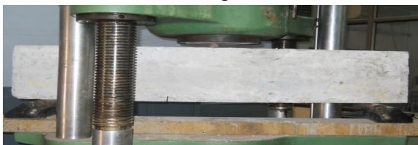
Fig: 4.17: M50-Large beam before Loading
