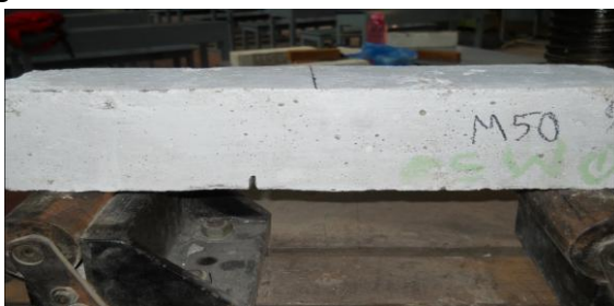
Fig.4.5: M50-Small beam before load
