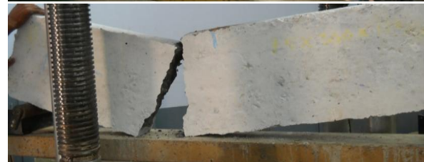
Fig: 4.13 & 4.14: M75-Large beam before Loading & after loading
