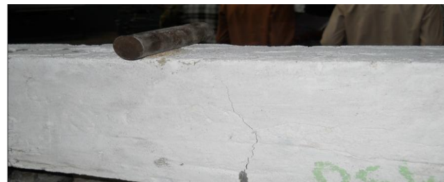
Fig.4.8: M50-medium beam after load
