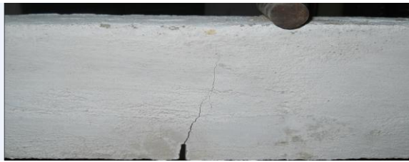
Fig.5.12: M75-medium beam after load
