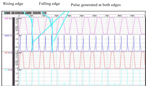
Figure. 7 waveform of Dual Edge triggered Sense-Amplifier
