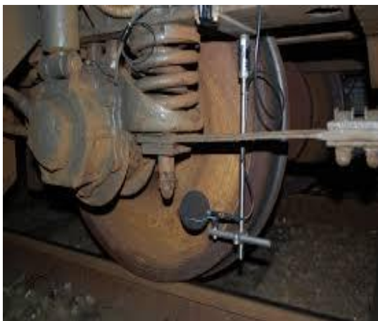
Figure 1.1: Model Figure to Fix the IR Sensor on the Wheel
