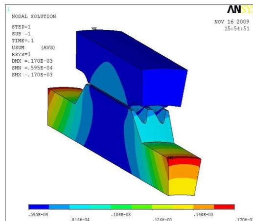
**Figure 3-1: 3D vector sum of deflection in the spline coupling from applied torque**
