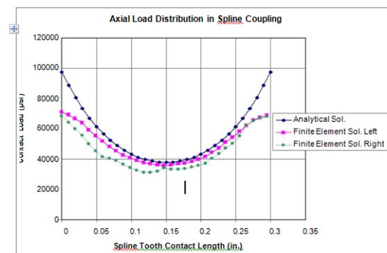
**Figure 3-4: Plot of contact pressure at root fillet radius verses contact length**
