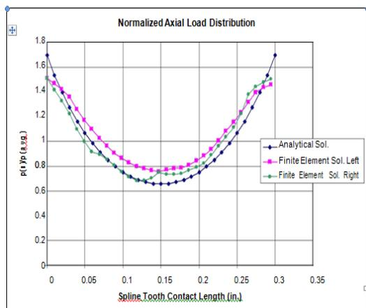
**Figure 3-5: Plot of normalized contact pressure,  $p(x)/p_{avg}$ , at the root fillet radius of the spline teeth versus contact length**
