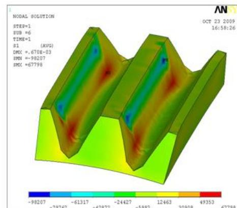
**Figure 3-3: Finite element model axial load distribution in the shaft spline teeth due to the applied torque**
