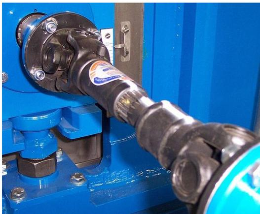
Fig 2.2 Power transmission through spline shaft
