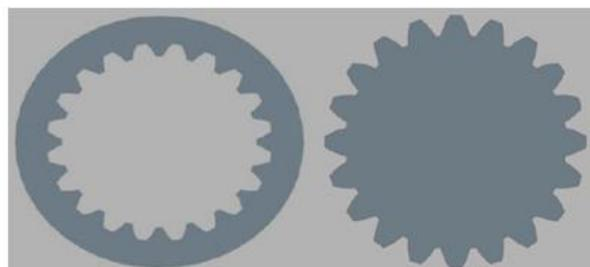
Fig 1.1 Sketch of Spline Shaft and Mating Shaft
