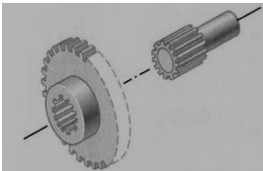
Fig 1.2 Schematic diagram of Spline shaft coupling system
