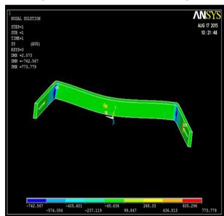
Fig.No.16. Stress distribution in the plate made of stainless steel Ti-6Al-4V (l=150 mm and t = 2.5 mm)
