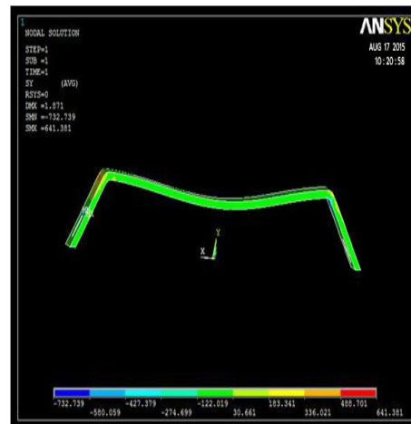
Fig.No.15. Stress distribution in the plate made of stainless steel Cr-Ni-Mo (l=150 mm and t = 2.5 mm)
