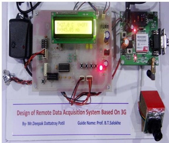
Fig.4: Complete Hardware of the system
