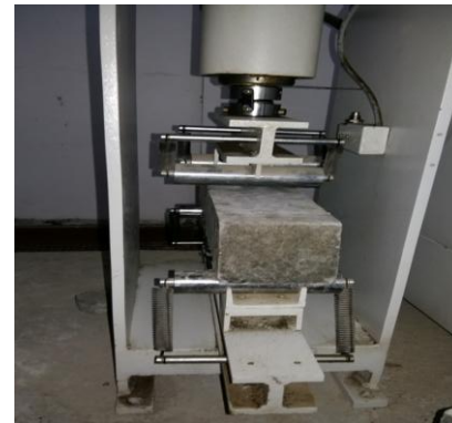
Fig 2. Test setup for flexural strength
