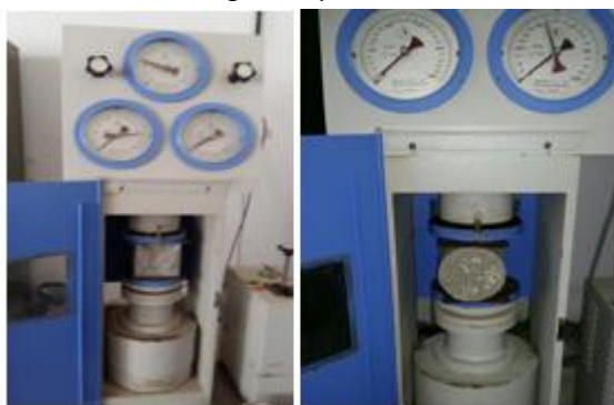
Fig 1. Test setup for compressive strength and split tensile strength respectively.
