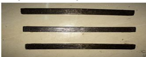
Fig: 2 A sample specimens after flexural test
