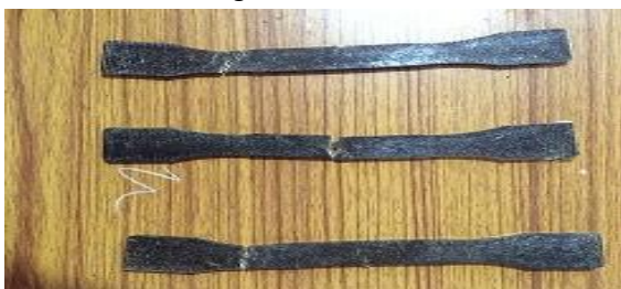
Fig: 1 A sample specimens after tensile test
