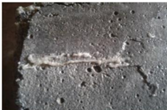
Figure 7- Crack healing in Sporosarcina globiospora after 28 days of compressive testing
