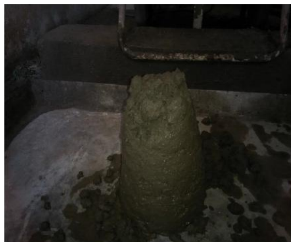
Figure 1- Slump value of approximately 100 mm
