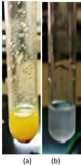
Figure 9- (a) Cured water sample with drops of concentrated hydrochloric acid, b) Effervescence due to change in color of sodium hydroxide.
