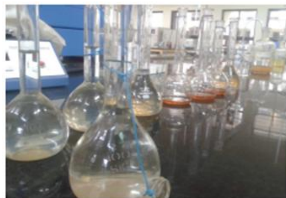
Figure 8- Comparison of color of test sample with standard ammoniac nitrogen solution
