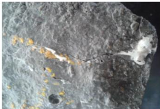
Figure 6- Crack healing in Bacillus subtilis after 28 days of compressive testing
