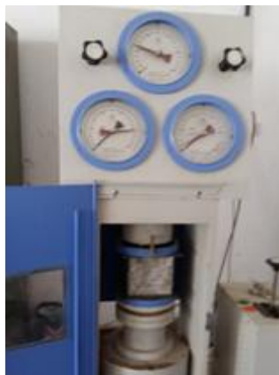
Fig-1: Test Setup for Compressive Strength Test
