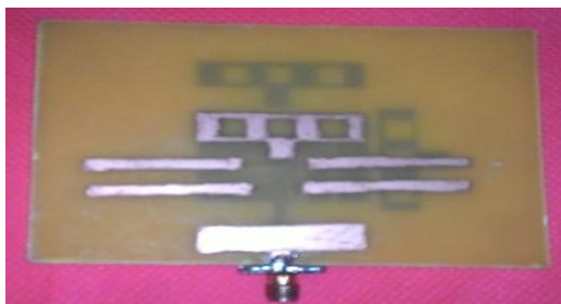
Fig. 11 Photograph for fabricated proposed antenna
