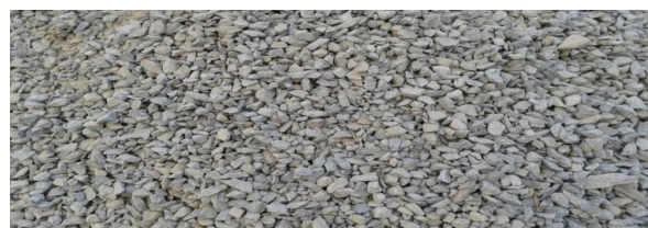
Fig 4.2: Locally available crushed aggregates
