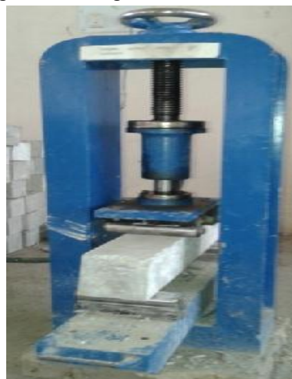
Fig 4.15: Flexural test on beams
