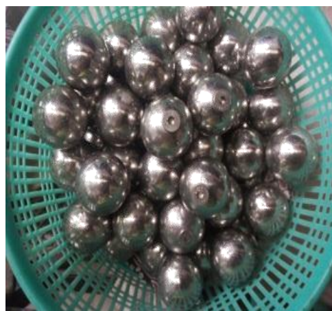
Fig2. PCM stainless steel capsule thermocouples set
