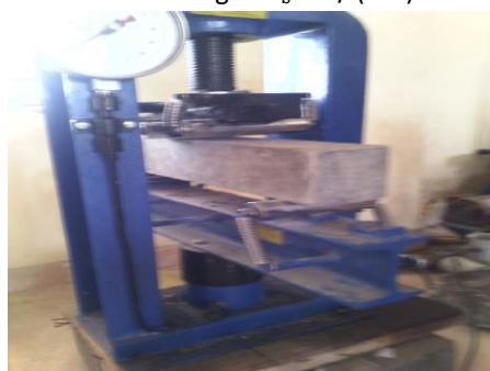
Fig 4 Flexural strength test set-up Split tensile strength test
