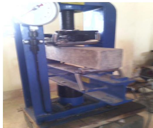
Fig 2 flexural strength test set-up
