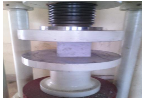
Fig 1 compressive strength test set-up Flexural Strength
