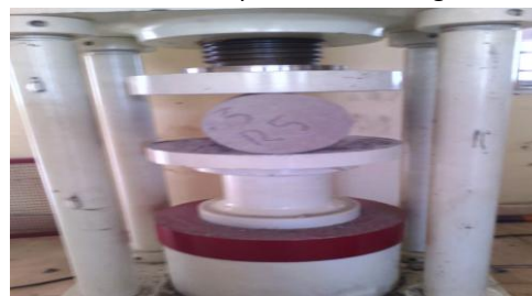
Fig 5 Split tensile strength test set-up
