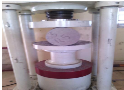
Fig 3 split tensile strength set-up
