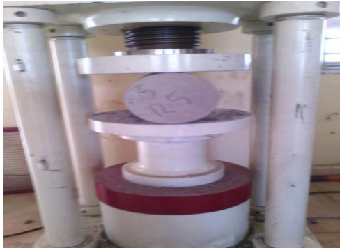
Fig 4 Split tensile strength test set-up
