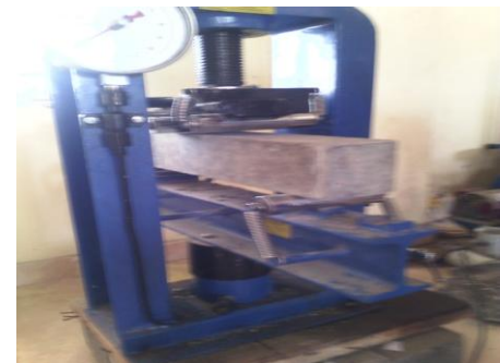
Fig 3 Flexural strength test set-up
