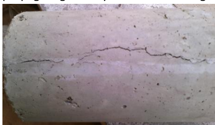
Fig 8 Crack Pattern of Cylinder
