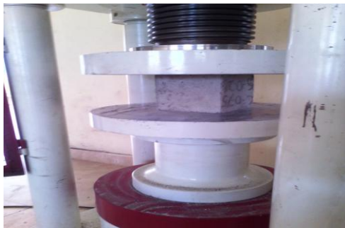
Fig 2 compressive strength test set-up
