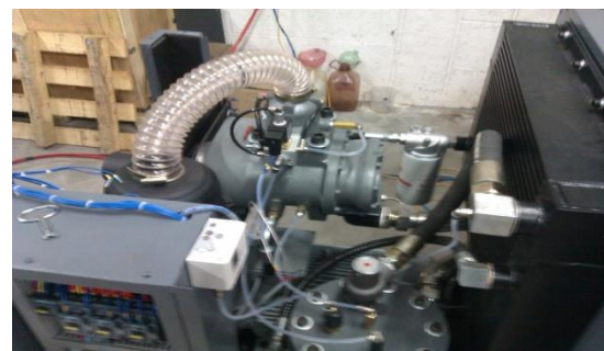
Figure 1 : Inside view of single screw compressor
