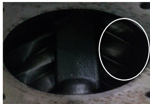
Figure 2: Occuring wear in starwheel
