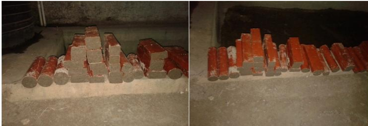
Fig-4: CFST Specimens immediate after casting.
