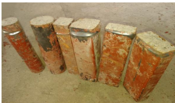
Fig-6: Failure Pattern of CFST Specimens
