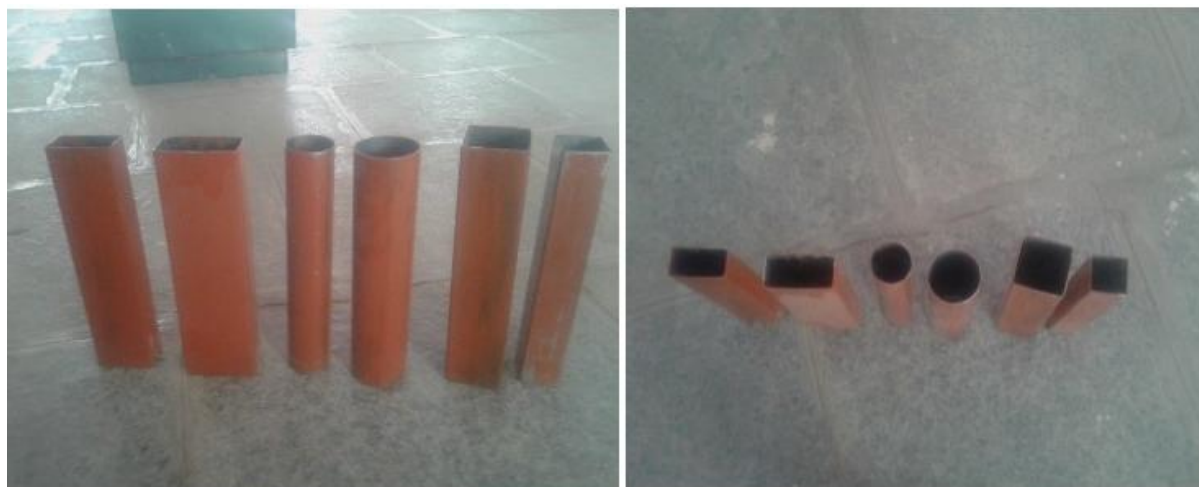
Fig-3: Steel tubes for casting of CFST specimens
