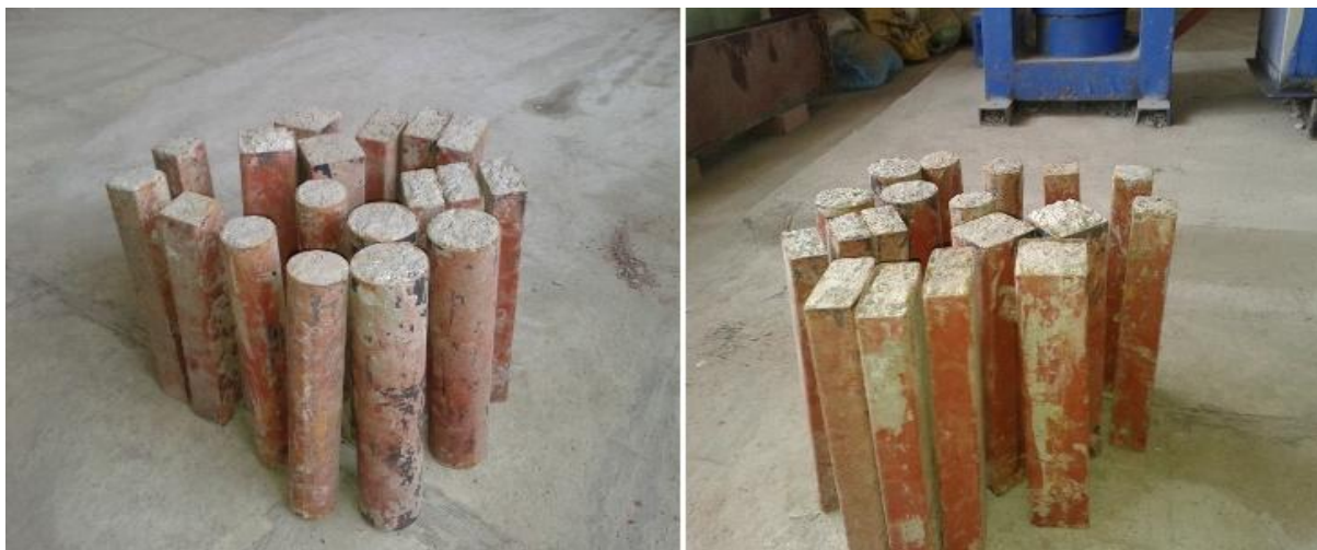
Fig-5: CFST Specimens after 28 days curing, before testing.
