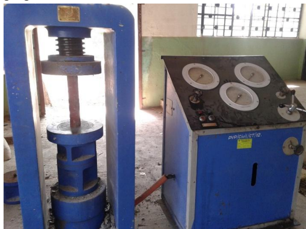
Fig-2: Photograph of Test setup for CFST on Compression Testing Machine.
