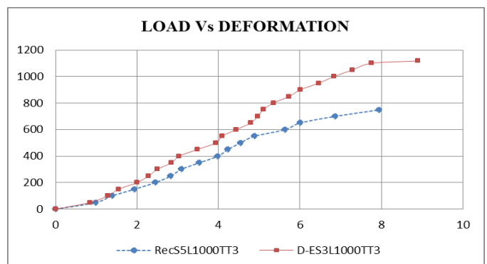
Figure 15 Axial load-deformation curves for RecS5L1000TT3 and D-ES5L1000TT3
