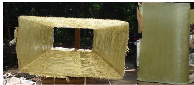
Figure1. Fabricated GFRP tubes
