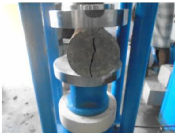
Fig 4: cylinder specimen at failure
