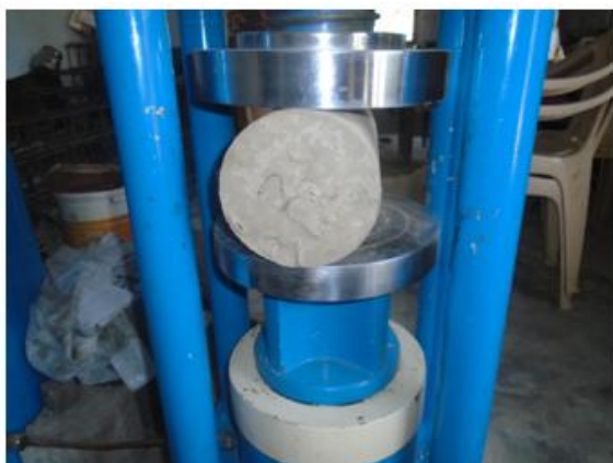
Figure 3 cylinder specimen setup
