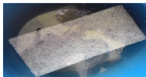
Fig- 8 brick immersed in water for efflorescence test
