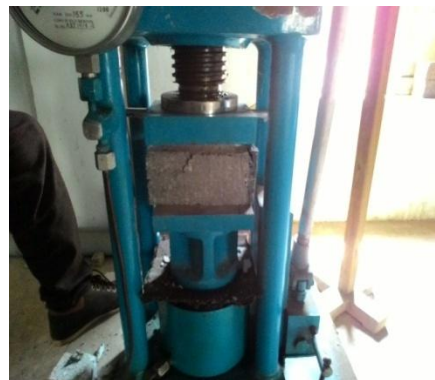
Fig – 7 performance of coqpressive strength test on Papercrete brick
