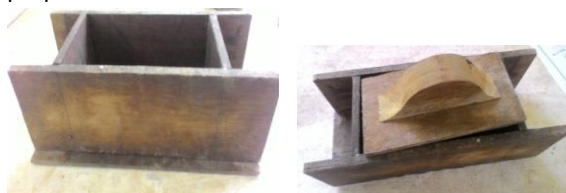
Fig – 5 Modular Brick Mould
