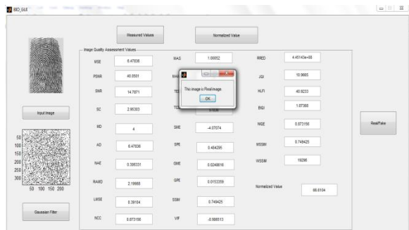
Fig 3: Image Quality Measures are calculated and Result of Real/Fake image for fingerprint
