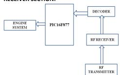
The receiver section is placed on the bike to control the ignition; it consists of an RF receiver, RF
