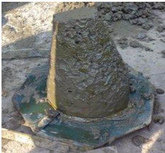
Fig.4 Slump cone test of scrap rubber
