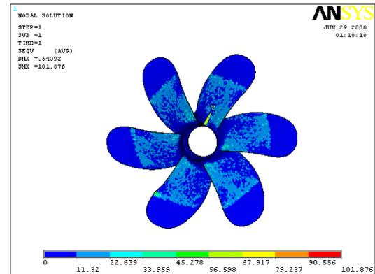
Figure 6.10: Max.von mises stress of composite propeller with 16 layers, MPa
