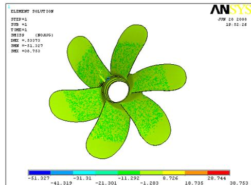
Figure 6.4: Max. von mises stress of composite propeller with 4 layers, MPa
