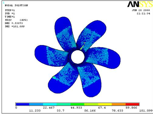
Fig 6.6: Max.von mises stress of composite propeller with 12 layers, MPa
