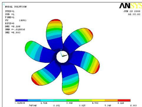
Figure 6.1: Max deflection of aluminum propeller, mm
