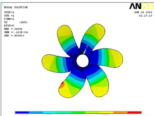
Figure 6.8: Max. deflection of composite propeller with 16 layers, mm
