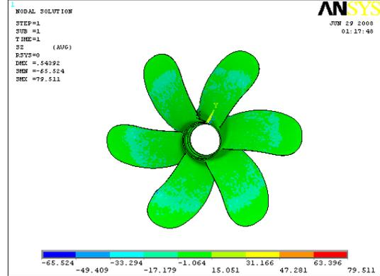
Figure 6.9: Max stress of composite propeller with 16 layers, MPa
