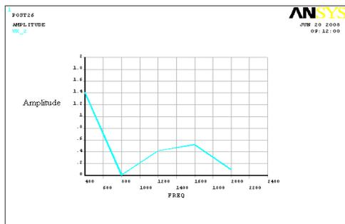
Figure 7: Frequency response of propeller made of aluminum material (in Ux direction)
