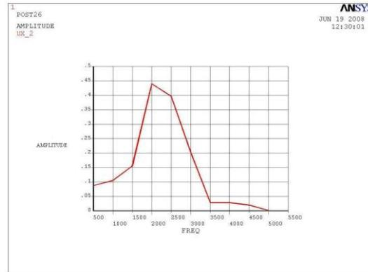
Figure 8: Frequency response of propeller made of composite material with 4 layers (in Ux direction)
