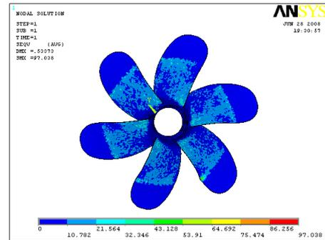
Figure 6.2 : Max. normal stress of composite propeller with 4 layers, MPa
