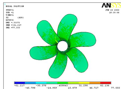
Figure 6.5: Max.inter laminar shear stress in composite propeller with 4 layers, MPa
