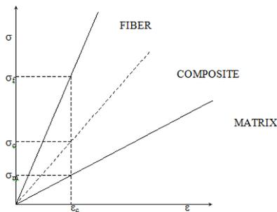
Figure.3.1 stress –strain diagram for a hypothetical composite material
