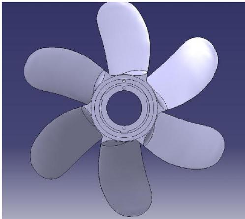
Figure 4: final solid model of propeller
