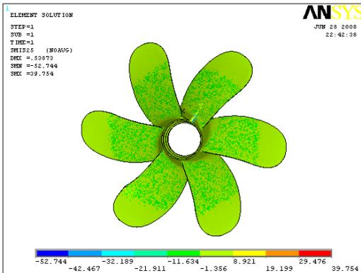
Figure:6.7 Max. Interlaminar shear stress of composite propeller with 12 layers, MPa
