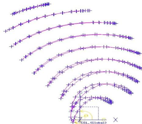
Figure 3. construction of hydrofoils by joining of points on surface of the blade
