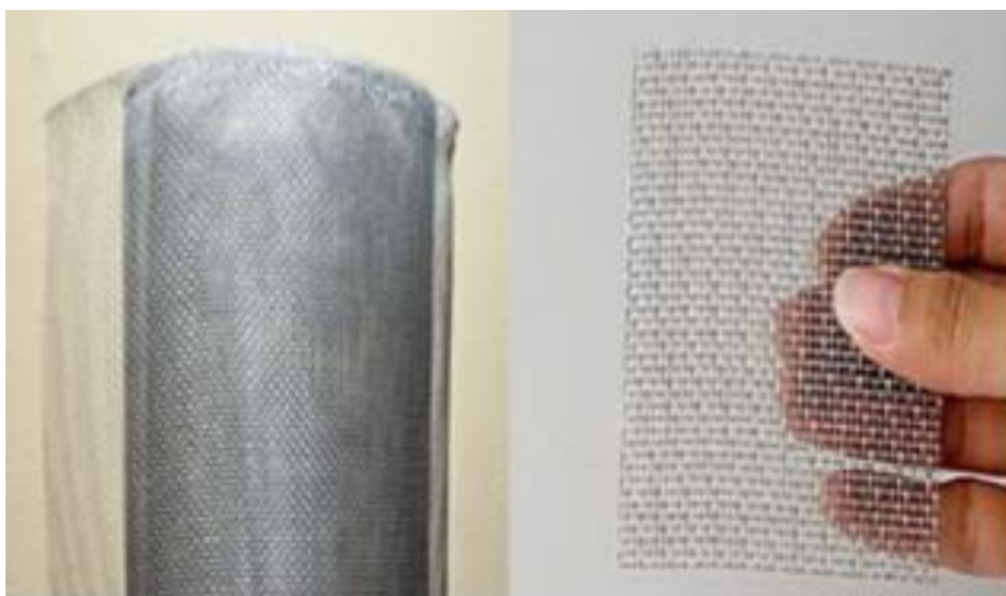
Fig .3 Screen mesh wick used in the heat pipe
