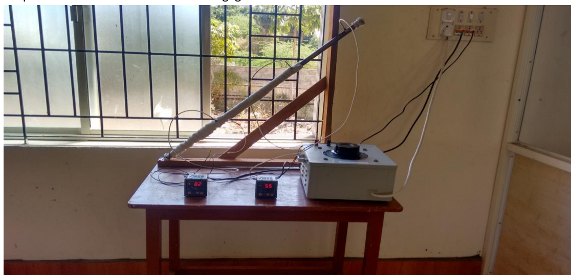
Fig 5. Heat Pipe Experimental Setup
