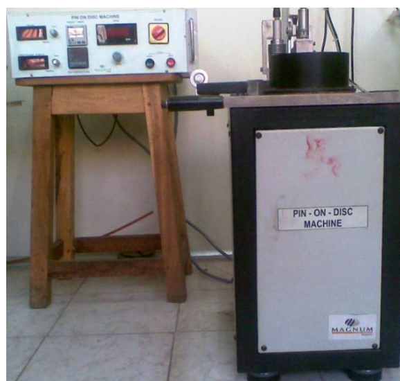
Fig.2.1:-set up to perform sliding wear on pin-on disc.
