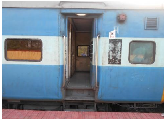
Fig 1: The floor to platform level in trains is at an uncomfortable level, even with the side handles and the gaps can be dangerous
