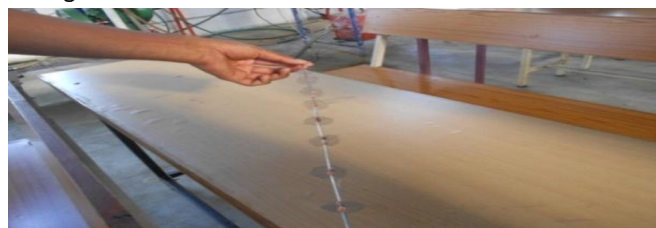
Fig5: photographic view of porous medium manufactured from iron screens. Mesh insert diameters along with different pitches
