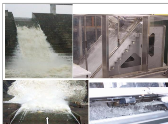
Figure 2. Prototype vs. laboratory stepped spillways (1V:0.8H): side-by-side comparison of aeration and energy dissipation [28].
